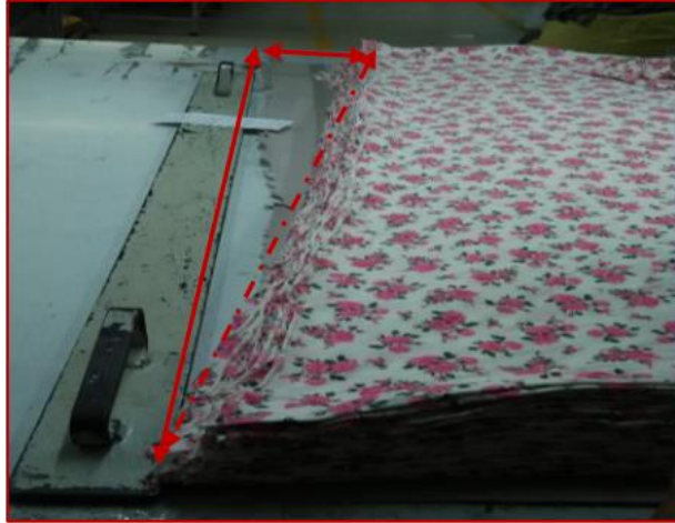
Skewing Observed Post Bit Washing
